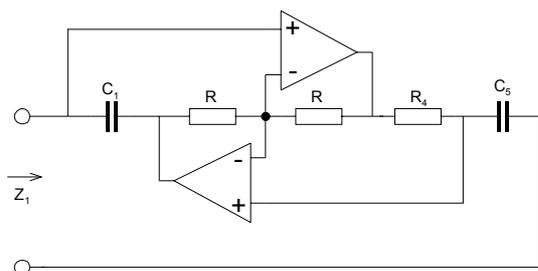
$$Z_1 = \frac{1}{sC_5} \frac{R \frac{1}{sC_1}}{RR_4} = \frac{1}{s^2 R_4 C_1 C_5} = \frac{1}{s^2 D} \quad (0-15)$$
