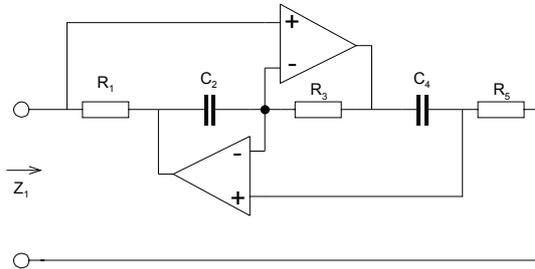
$$Z_1 = R_5 \frac{R_1 R_3}{\frac{1}{sC_2} \frac{1}{sC_4}} = R_1 R_3 R_5 s^2 C_2 C_4 = s^2 N \quad (0-16)$$
